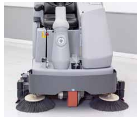
Retractable side brooms on cylindrical models sweep debris away from pallets
