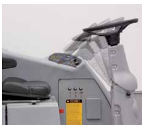
Tilt steering wheel for easy boarding, plus ergonomically designed operator compartment for safety and comfort
