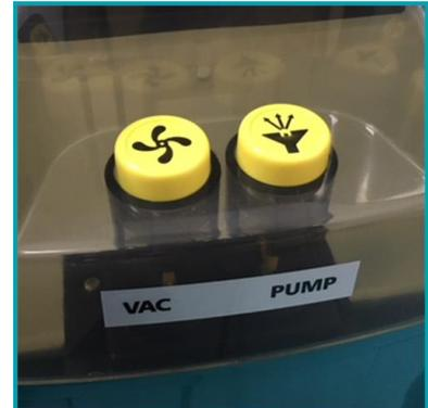
Switch on the pump spray and/or vacuum.
