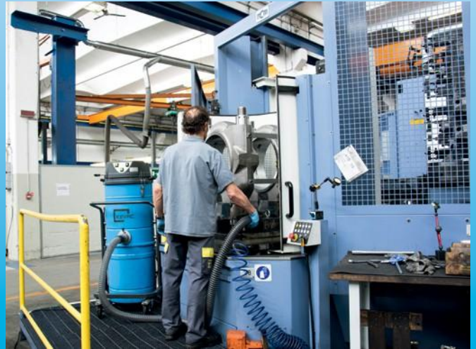
Swarf removal from lathe
