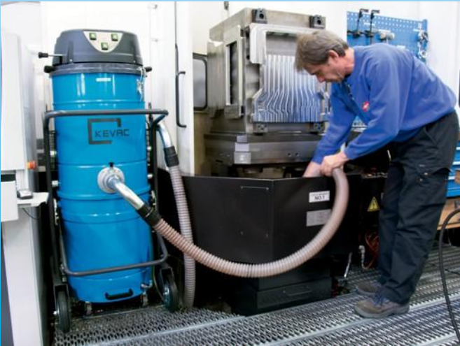
Working station cleaning operation on multi station milling machine
