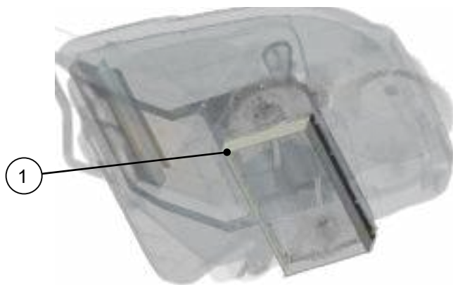
1 dust guard rubber blades for the central brush
