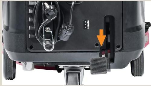
Lift the deck by pressing the pedal
